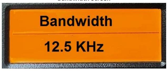
If the voice was enabled, then the radio will annunciate "Bandwidth" followed by "12.5 Kilohertz" or "25 Kilohertz"
