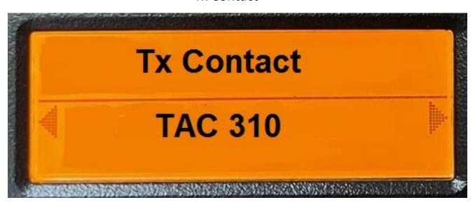
If the voice was enabled, then the radio will annunciate "Tx Contact" followed by the annunciation of Line 2 on a character by character basis.
