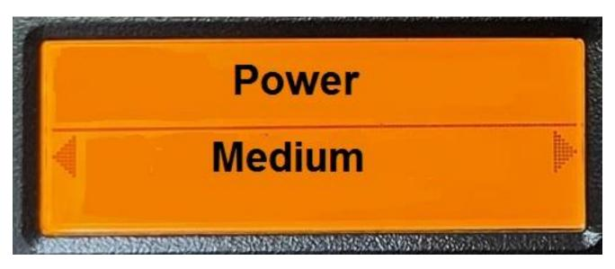
If the voice was enabled, then the radio will annunciate "Power Low", Power Medium", or "Power High"
