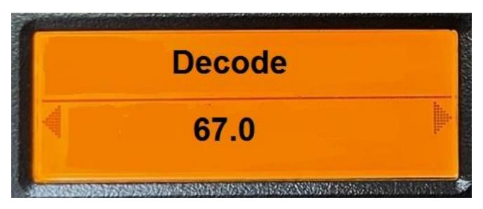
If the voice was enabled, then the radio will annunciate "Decode" followed by the value of the CTCSS or DCS.
