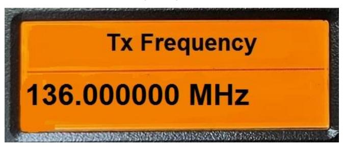
If the voice was enabled, then the radio will annunciate "Tx Frequency" followed by the value of the frequency followed by MHz.
