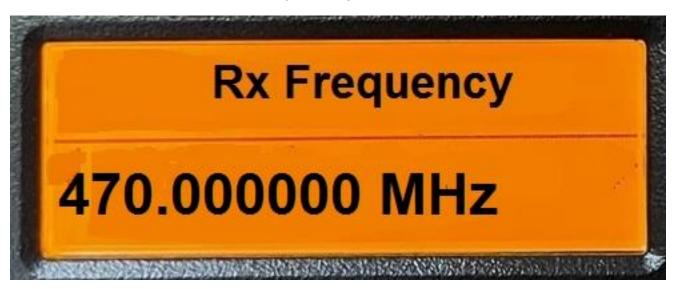
If the voice was enabled, then the radio will annunciate "Rx Frequency" followed by the value of the frequency followed by MHz
