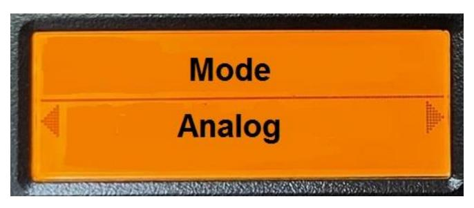
When the Enhanced Parameter mode is first selected, the screen above will appear. Depending on the value of the current channel selected in the radio, the second line is going to show "Analog" or "Digital".
