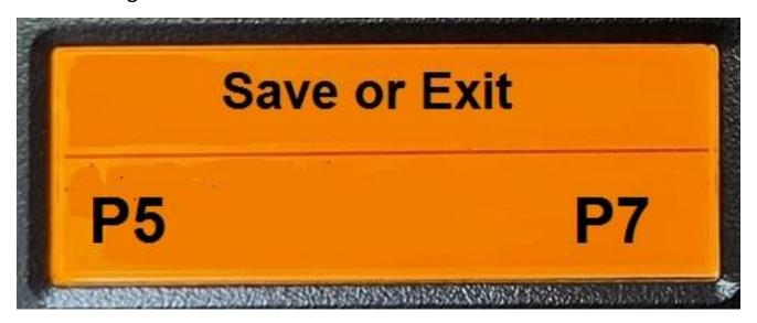
If you pressed the P1 key, then you will want to permanetly save the updated channel in the currrent channel. You will replace the original channel and exit from this routine. Turning off the radio or changing channels will not erase this channel.
