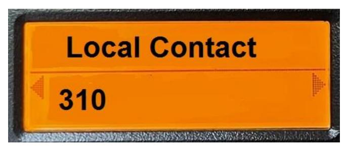
If the voice was enabled, then the radio will annunciate "Local Contact" followed by the value of the contact.
