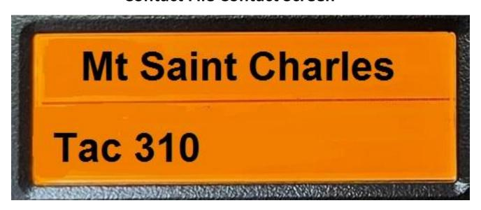
If the voice was enabled, then the radio will annunciate "Contact File Contact" followed by the annunciation of line 2 on a character by character basis.
