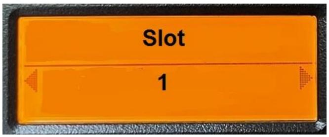
If the voice was enabled, then the radio will annunciate "Slot" followed by the value of the Slot
